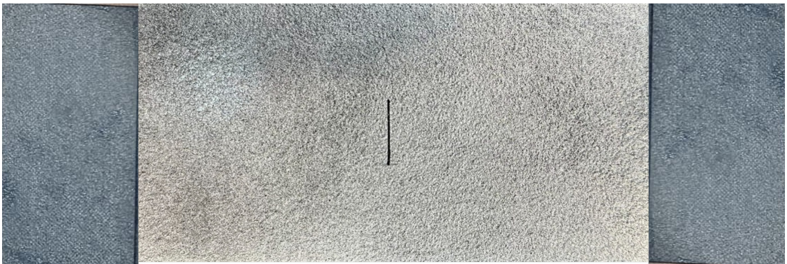
Figure 2.2 Representative front surface preparation of the pre-cracked composite laminate specimen with a random black-and-white speckle pattern used for digital image correlation measurements.
